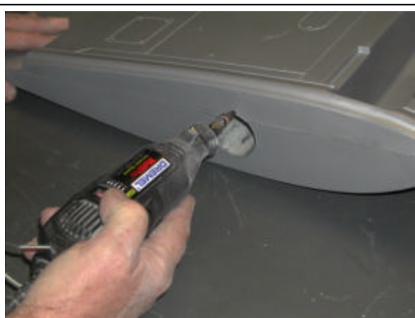
Using a dremmel tool, notch a hole 1/8 inch deep in the underside of the wing on one side. This will allow the bolt head to lock in place. Make sure that this a tight fit.
