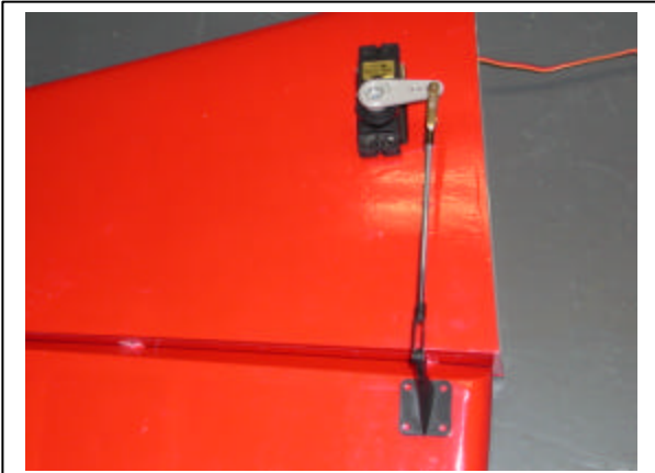
Completed stab half with elevator linkage.
