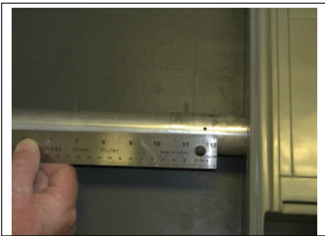
11 5/8 inches from the end of the tube. Drill and tapped hole.
