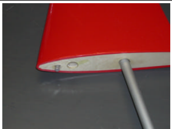
Epoxy the anti rotation pin and epoxy the stab tube into only one half of the stab at this time. We will glue the other half in later.
