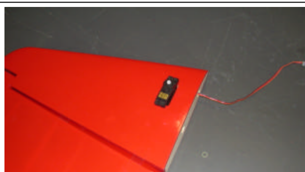
Completed stab half with servo installed
