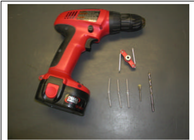
These are the tools for the proper installation of the hinges in the elevators, rudder and ailerons.
