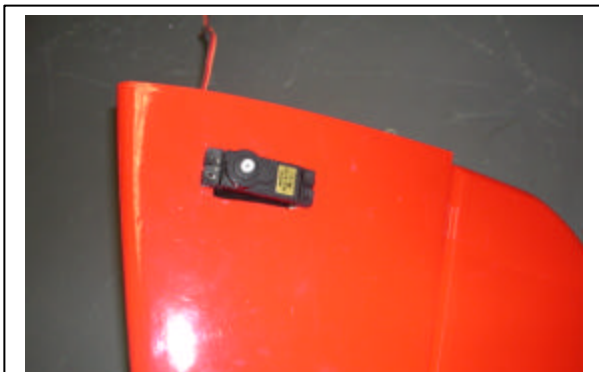
Remove covering for the servo and check the pocket for clearance for the servo wife.
