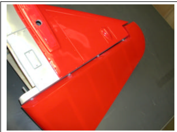
The rudder is install using four hinges. The procedure is much the same as used for the ailerons and elevators.
